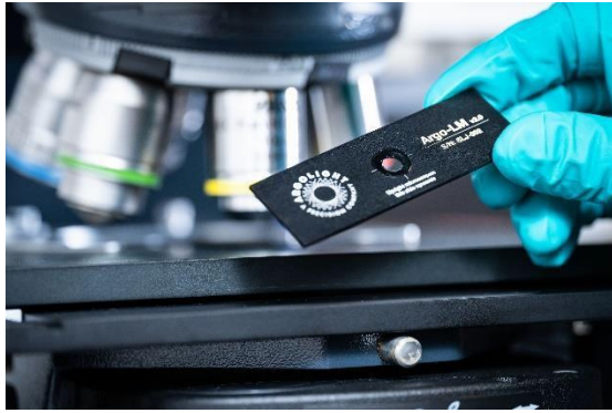
Figure 1: An Argolight QC slide
