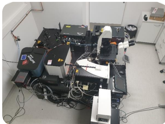
Figure 1 : CARS and multiphotonic spectro-microscopy system
